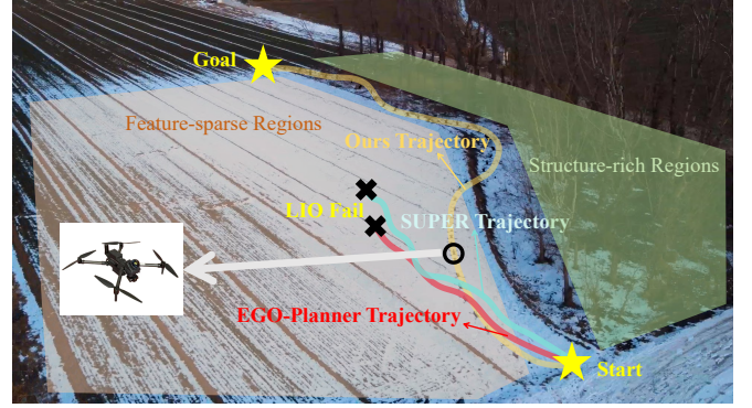
Fig. 1. Real-world illustration of the motivation and function of AUG in long-range GNSS-denied navigation. Although the direct route from start to goal is geometrically feasible, the open field is a feature-sparse region in which LiDAR-inertial odometry (LIO) is prone to degeneration, while the tree-lined boundary provides a structure-rich region with more informative constraints for LIO. As a result, baseline planners ( EGO-Planner in red and SUPER in cyan) enter the feature-sparse area and fail due to localization degradation (black crosses), whereas AUG (yellow) selects a perception-aware route through the structure-rich corridor to maintain estimator conditioning and reach the goal reliably.
